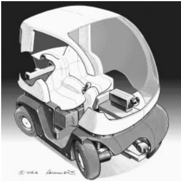
Figure 1: Semi Autonomous Electrical Vehicle: The CyCab
